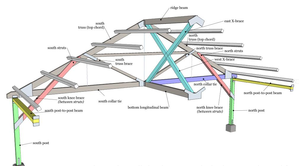
**NOTE:** There are eight trusses like this in the structure, named T1 through T8, starting at the west end of the pier. Each component of the structure can be uniquely identified using these names.
